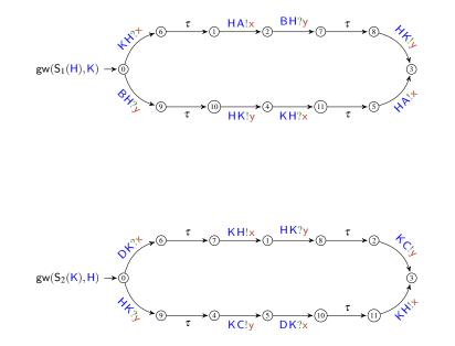
The composed system  $S_1 \stackrel{H \leftrightarrow K}{\to} S_2$  deadlocks when  $gw(S_1(H), K)$  receives from B while  $gw(S_2(K), H)$  receives from D since both gateways reach an output state (respectively states 10 and 7).
