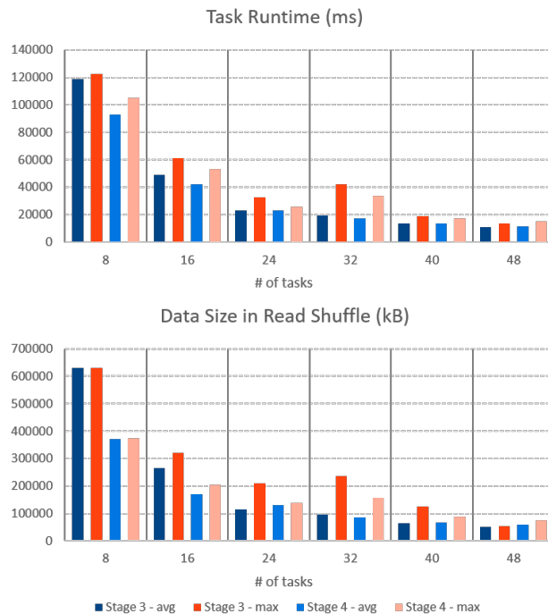
Fig. 1. The skew in partitioned data (i.e., data shuffled from previous stage and read by each task as a part of its input) and its impact on task execution times: We report the total size of shuffled data and task execution times in stages 3 and 4 when running PageRank application with 2.8 GB of data on Spark cluster of 4 nodes, deployed in Rennes site of Grid'5000. The number of stages is set to 6 stages.
