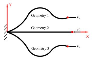
Figure 2: Nonlinear buckling of a slender straight beam
