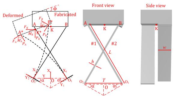
Figure 25: Constitutive, force equilibrium and compatibility relationships of a straight-beam-based cross-axis compliant revolute joint and its schematic geometry
