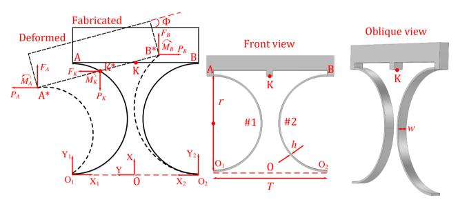
**Figure 36:** Constitutive, force equilibrium and compatibility relationships of a circular-beam-based compliant revolute joint and its schematic geometry
