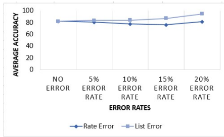
Fig. 8. Accuracy of leakage detection in all nodes
