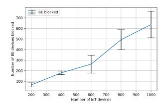
(b) Number of blocked IoT devices from the low priority slice for a target PDR=90%
