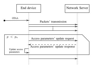
Fig. 2: Update request/response communication between the end device and the network server.
