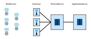
Fig. 1: LoRaWAN architecture.
