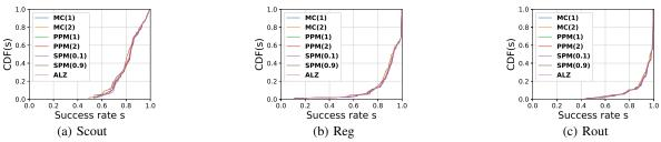
Fig. 4: Distribution of the success rate score  $s_{\mu}$  of each predictor per profile for the Agg\_gps dataset.
