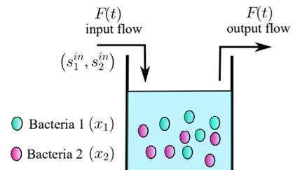
Fig. 1. Continuous stirred tank bioreactor with two bacteria.
