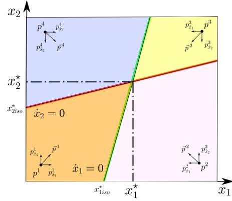
Fig. 3. Direction of the trajectories  $\bar{p}^i$  for possible initial conditions  $p^i$ , nullclines ( $\dot{x}_1 = 0, \dot{x}_2 = 0$ ), isolated equilibria ( $x_{1,iso}^*, x_{2,iso}^*$ ) and intersection.
