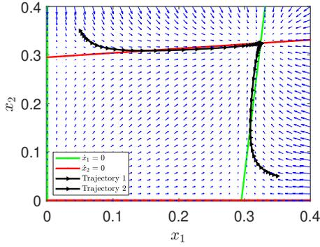
Fig. 4. Phase portrait of the bacteria ( $x_1 - x_2$ ) for Example 1, nullclines for  $\dot{x}_1 = 0$  and  $\dot{x}_2 = 0$  are indicated in green and red, respectively. Trajectories from simulation with initial conditions (0.05, 0.35) and (0.35, 0.05).
