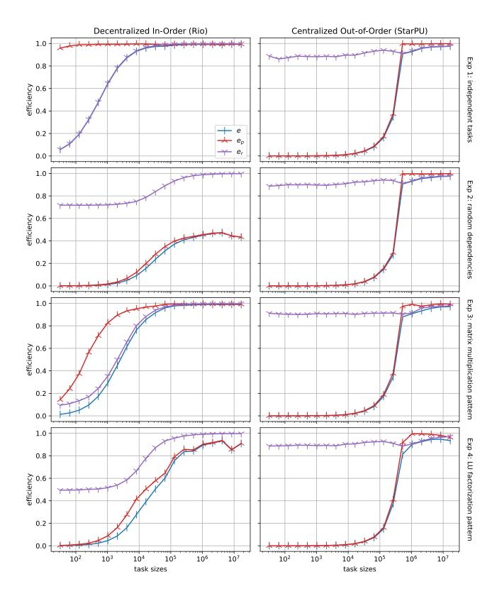
Fig. 8. Efficiency decomposition as a function of task sizes for a decentralized in-order runtime (R10) and a centralized OoO runtime (StarPU) on different task graphs.
