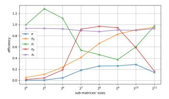
Fig. 4. Efficiency decomposition on a 4096 by 4096 square matrix multiplication with StarPU (24 threads).
