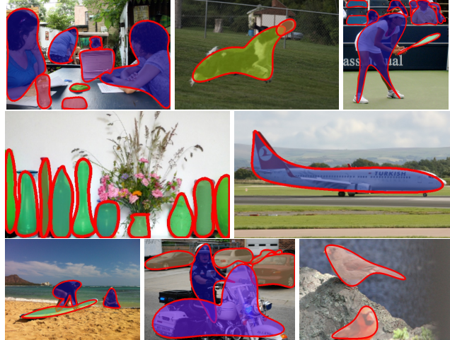
Figure 1. Our algorithm captures the silhouette of objects with a compact resolution-independent representation based on Fourier coefficients. Contours produced by our algorithm adequately approximate the general shape of free-form objects such as persons, animals, cars or pots while being defined in a simple parametric way with only a few complex Fourier coefficients, here 8. Images from COCO 2017 test-dev.
