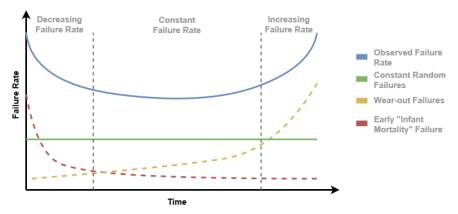
Fig. 1 The bathtub curve describing the failure rate of electronic circuits over their lifespan [39]
