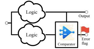
**Fig. 3** Generic structure of the *duplication with comparison* architecture.
