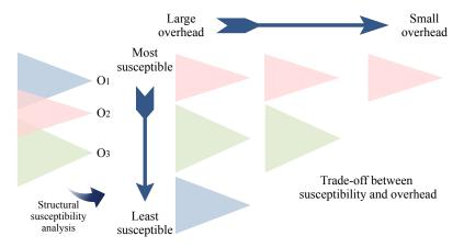
Fig. 13 Reduced duplication scheme based on structural susceptibility analysis
