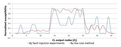
Fig. 12 Comparison of the structural susceptibility analysis and a fault injection experiment, for the b03 circuit from the ITC'99 benchmark suite. Taken from [14]
