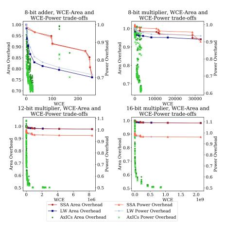
Fig. 15 Experimental results comparing the four scenarios: reduced duplication based on the structural susceptibility analysis (SSA); reduced duplication based on the logical weights of the arithmetic circuit outputs (LW); reduced duplication scheme based on an approximate arithmetic circuits from [47] (AxICs)
