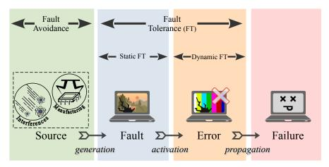
Fig. 2 Reliability improvement approaches across the fault-to-failure life cycle [10]
