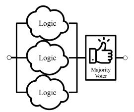
**Fig. 4** Generic structure of the Triple Modular Redundancy architecture.
