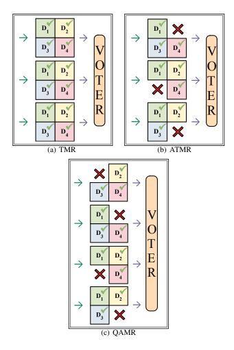
**Fig. 16** (a): three identical copies are used in TMR: all produce the correct results for all the function's domains (D1-D4) when no errors occur. — (b): in ATMR approach the three approximate modules produce exact results only for three out of four function's domains; some domains are not covered three times as in the TMR scheme. — (c) QAMR approach: four approximate modules cover each function's domain three times, thus obtaining the same coverage as in the TMR scheme.
