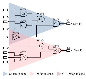
Fig. 11 Example of structural susceptibility analysis application to a simple circuit.
