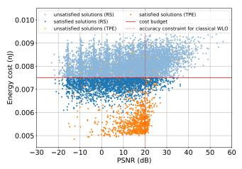
Fig. 2: The classical WLO problem in the context of the cost-constrained WLO problem. The data points includes the 10000 randomized solutions and 1000 solutions found by TPE for the classical WLO problem with an accuracy constraint as 25 dB of PSNR.
