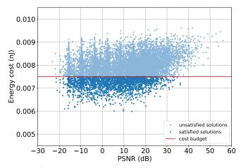
Fig. 1:  $10^5$  random solutions as a representative subset of all possible solutions, for the FIR filter benchmark. The red line represents an energy budget of 0.0075 nJ
