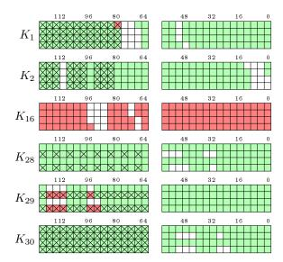
Fig. 7: Determining all the active keybits for all approximations (crossed out in the figure) with as few guesses as possible. We can deduce the (light) green bits if we know the 123 keybits highlighted in (dark) red.
