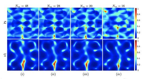
Figure 4: Time- vs. frequency- domain inversion from reduced data at 60% of the maximum load: (top) multifrequency indicator  $\mathfrak{L}$  [23], and (bottom) time-domain indicator  $\mathfrak{T}$ . Here, the number of scanning points on  $\Gamma_m$  is  $N_m$ .
