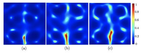
Figure 1: Time-domain reconstruction of an advancing fracture: (a-c)  $\mathfrak{T}$  maps computed from ultrasonic waveforms measured at 90%, 75%, and 60% of the maximum load in the post-peak regime. The solid line shows the ground truth.
