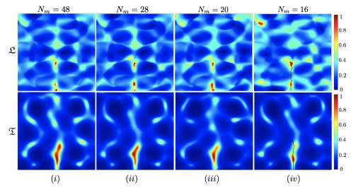
Figure 4: Time- vs. frequency- domain inversion from reduced data at 60% of the maximum load: (top) multifrequency indicator  $\mathfrak{L}$  [22], and (bottom) time-domain indicator  $\mathfrak{T}$ . Here, the number of scanning points on  $\Gamma_m$  is  $N_m$ .
