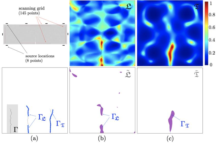
Figure 2: Time- vs. frequency- domain reconstructions from post-fracturing data: (a-top) sensing configuration, (a-bottom) ground truth  $\Gamma$  compared against the recovered  $\Gamma_{\Xi}$  and  $\Gamma_{\Xi}$  obtained from the thresholded maps, (b) multifrequency indicator map  $\Xi$  and its 60% thresholded counterpart  $\tilde{\Xi}$  [22], and (c) time-domain indicator map  $\Xi$  (6.24) and its affiliated  $\tilde{\Xi}$  (6.25) thresholded at 60%.
