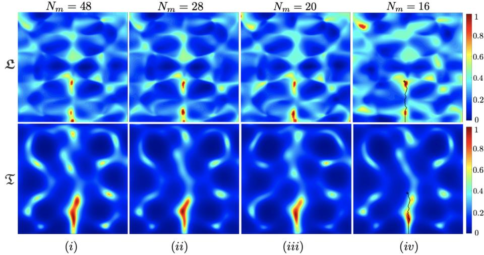
Figure 4: Time- *vs.* frequency- domain inversion from reduced data at 60% of the maximum load: (top) multifrequency indicator  $\mathfrak{L}$  [22], and (bottom) time-domain indicator  $\mathfrak{T}$ . Here, the number of scanning points on  $\Gamma_m$  is  $N_m$ .
