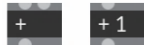
Fig. 16 The “+” function has two inlets by default, one will be suppressed by adding an argument
