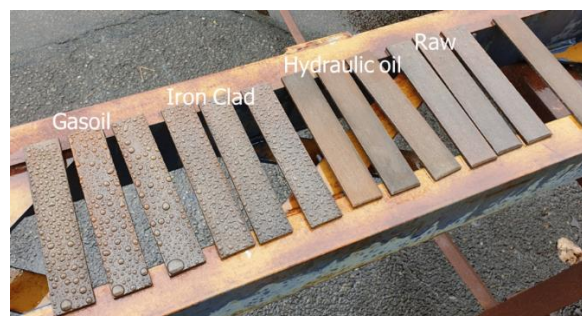
Figure 1: SPECIMENS USED FOR THE SURFACE PREPARATION ANALYSIS AFTER AGEING AND POLLUTION.
