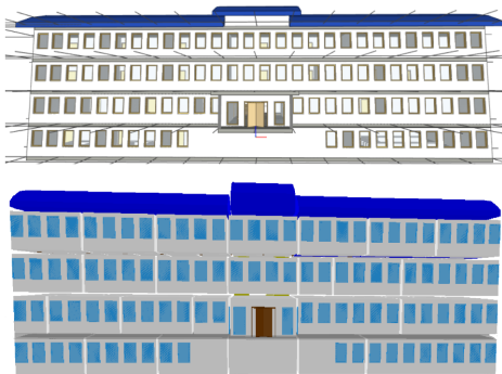
Figure 12: IFC building visualised using BimVision (above) vs. NGSI-LD visualization using python trimesh (below)
