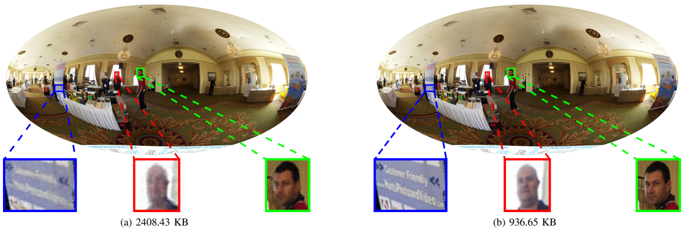
Fig. 16. Decompressed images in Mollweide projection. The zoomed versions of red, green, and blue rectangular regions are shown in the bottom row. (a) DeepSphere result stored in 2408.43 KB with 29.54 dB and 29.51 dB for SPSNR and WSPSNR respectively. (b) OSLO result stored in 936.65 KB with 40.91 dB and 41.65 dB for SPSNR and WSPSNR respectively.
