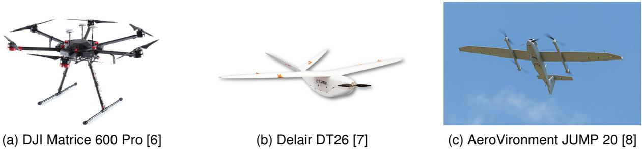
Figure 1 – Multicopter, Fixed-Wing and FW-VTOL concepts
