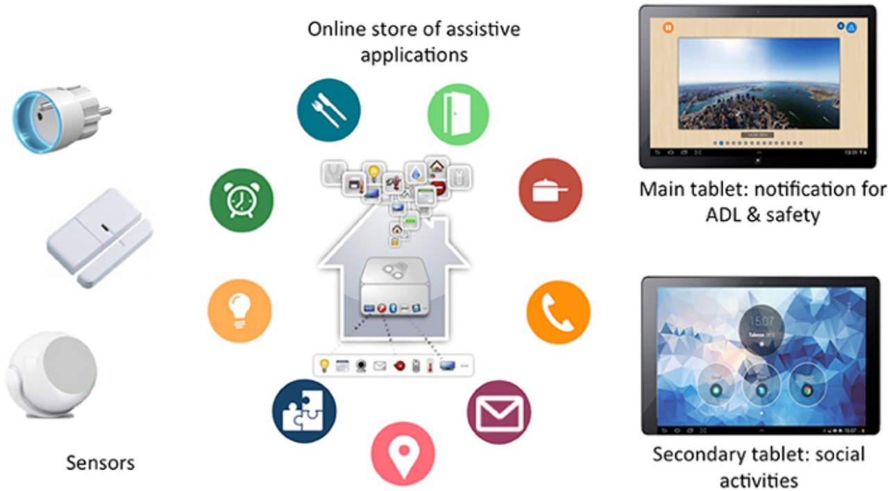
Figure 2. Content of HomeAssist platform—a set of sensors, a web-based catalog of assistive applications, and two touch screen tablets (main and secondary). ADL: activities of daily life.
