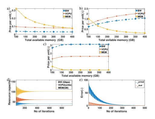
Fig. 4. Changes in the price ( $\lambda$ ) with respect to the available memory capacity, with a)  $\rho = 0.1$ , b)  $\rho = -1.5$ , and c)  $\rho = -2.5$ . d) Convergence of Algorithm 3, convergence of total resources' demand to the available capacity. e) Convergence of the primal and dual errors in Algorithm 3.
