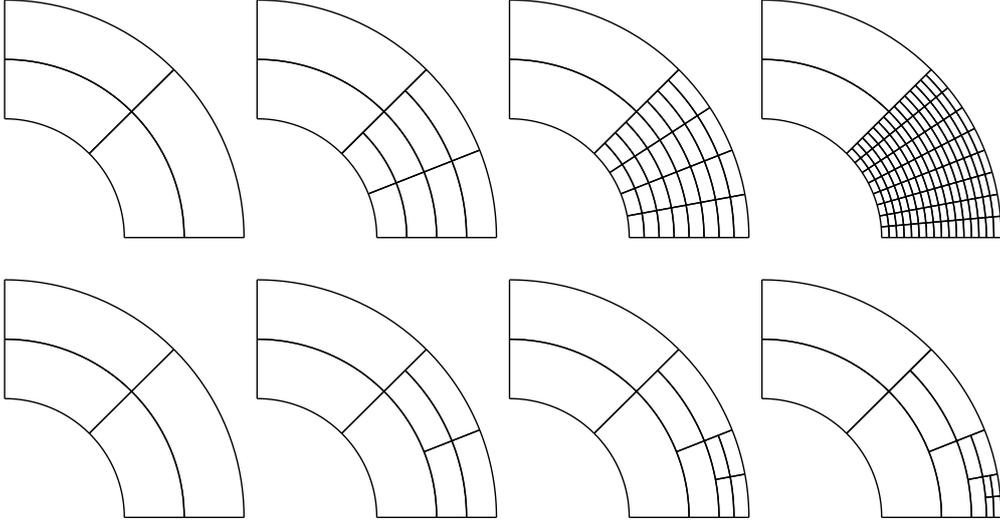
FIGURE 7. The domain  $\Omega$  considered in Section 9 along with the initial mesh  $\mathcal{T}_0$  and the first three refinements: in the right half of  $\Omega$  (leading to arbitrary many hanging nodes) (top) and towards the point  $(1, 0)$  (violating the bounded patch overlap condition (84a)) (bottom).
