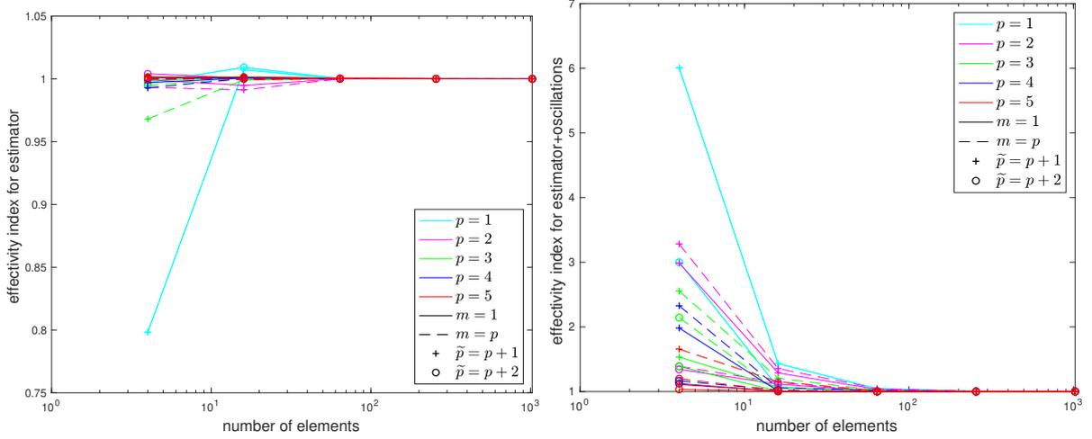
FIGURE 8. Effectivity indices  $\frac{\|\sigma_h + \nabla u_h\|_{\Omega}}{\|\nabla(u - u_h)\|_{\Omega}}$  (left) and  $\frac{\|\sigma_h + \nabla u_h\|_{\Omega} + \text{osc}_h^{\text{rel}}}{\|\nabla(u - u_h)\|_{\Omega}}$  (right) corresponding to the problem of Section 9 with uniform mesh refinement, polynomial degrees  $p \in \{1, \dots, 5\}$ , multiplicities  $m \in \{1, p\}$ .
