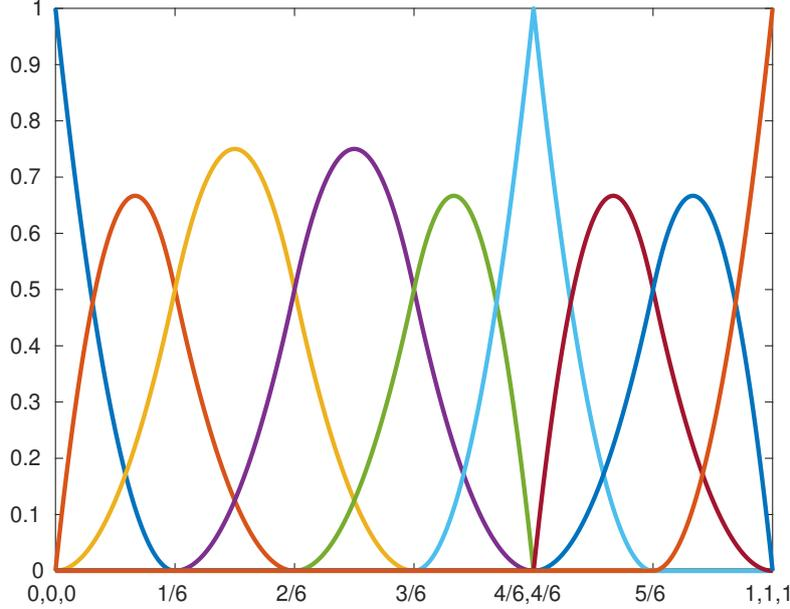
FIGURE 4. The B-splines of degree  $p = 2$  corresponding to the knot vector  $\mathcal{K} = (0, 0, 0, 1/6, 2/6, 3/6, 4/6, 4/6, 5/6, 1, 1, 1)$  are depicted. They are at least  $C^1$  at the knots  $1/6, 2/6, 3/6,$  and  $5/6$ , and at least  $C^0$  at  $4/6$ .
