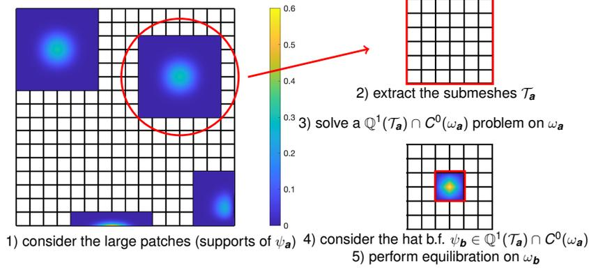
FIGURE 3. Inexpensive equilibration in IGA in the simplified setting of uniform tensor-product mesh,  $p = 5$  and maximal smoothness  $p - 1$ .
