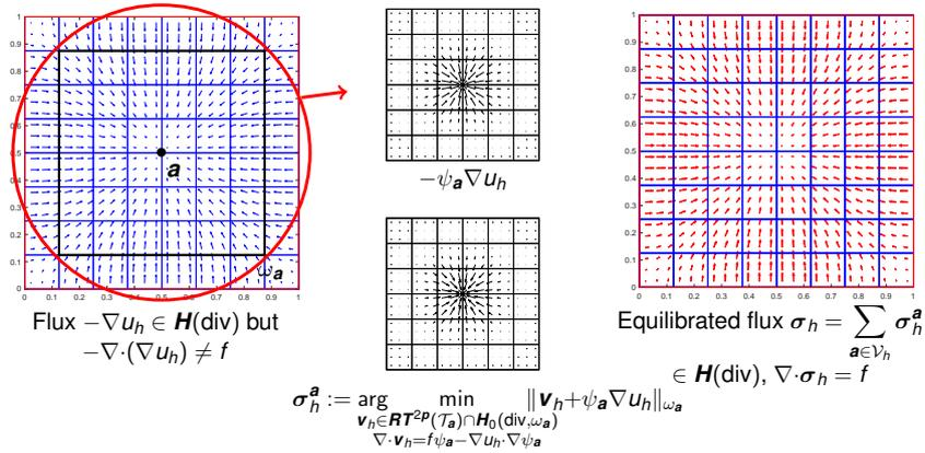
FIGURE 2. A straightforward (expensive) extension of the FEM equilibration to IGA with B-splines of degree  $p = 5$  and maximal smoothness  $p - 1$  on a two-dimensional uniform tensor mesh  $\mathcal{T}_h$ .
