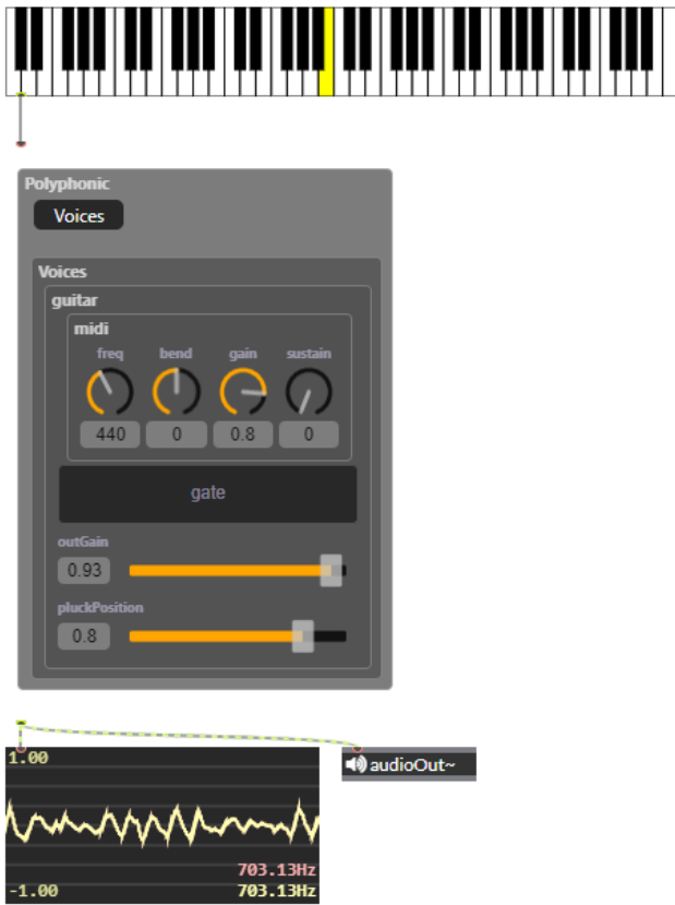
Figure 4: A Faust polyphonic WAM generated by faust2wam and loaded in JSPatcher, connected with a virtual keyboard and an oscilloscope.
