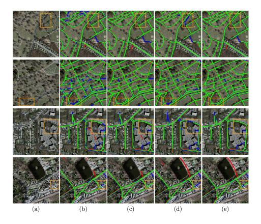
**Fig. 7.** Segmentation results from the Massachusetts dataset: green represents true positive (TP), red represents false positive (FP), blue represents false negative (FN). (a): Original image; (b): ResUnet; (c): ResUnet+CUnet; (d) D-LinkNet; (e) D-LinkNet+CUnet.
