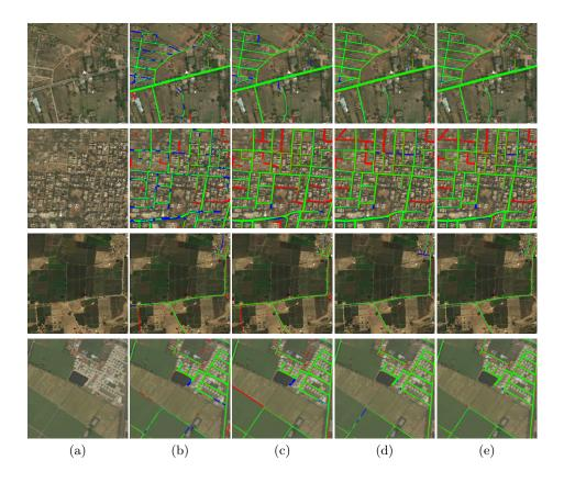
**Fig. 8.** Segmentation results from the DeepGlobe dataset: green represents true positive (TP), red represents false positive (FP), blue represents false negative (FN). (a): Original image; (b): ResUnet; (c): ResUnet+CUnet; (d) D-LinkNet; (e) D-LinkNet+CUnet.
