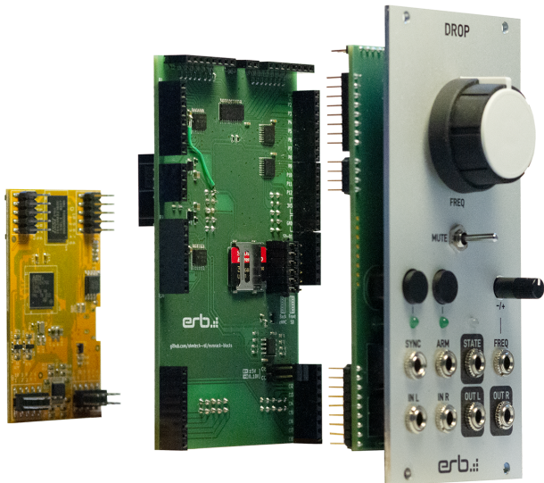
Figure 5: From left to right, the Daisy Patch Submodule board, the Eurorack-block board "Kivu12", the front PCB tightened to the front aluminum panel with its jack connectors and pot.
