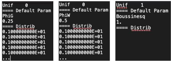
**Figure 12**: *DIP\_cell\_porosity\_map.txt* (left), *DIP\_edge\_porosity\_map.txt* (middle) and <u>Boussineq\_map.txt</u> (right) files for the DIP simulation of the Sacramento test case. The two first files are partially presented, since they contain values for all cells and edges, respectively (*Unif* is set to 0, so the default value is ignored). The third file is fully presented.
