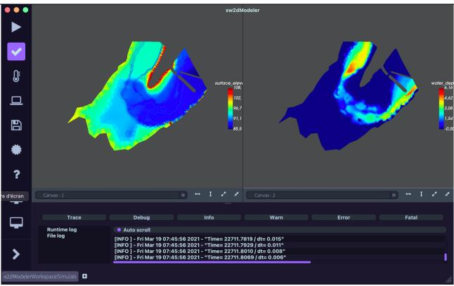
**Figure 9**: Visualization in the SW2D GUI of results obtained for Gardon test case near the beginning of the flood pic. Left: surface elevation (the ground elevation is displayed when there is no water in the cell). Right: water depth.
