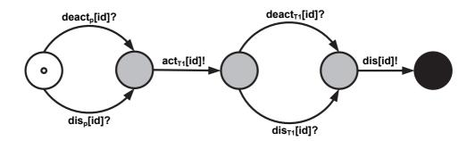
Figure 12. STA template for DRBD SPARE block.
