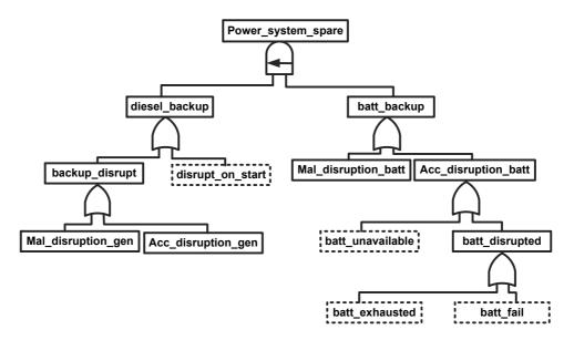
*Figure 7.* Power\_system\_spare AFT. The leaves drawn with black and bold lined rectangle represents a malicious failure. The leaves drawn with light black and dashed lined rectangle represents an accidental disruption.
