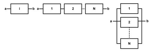
Figure 2. Standard RBD configurations (from left to right): a block representing the functional system component  $C_i$  with end points **a** as the input and **b** as the output, Series configuration with N number of blocks and Parallel configuration with N number of blocks.
