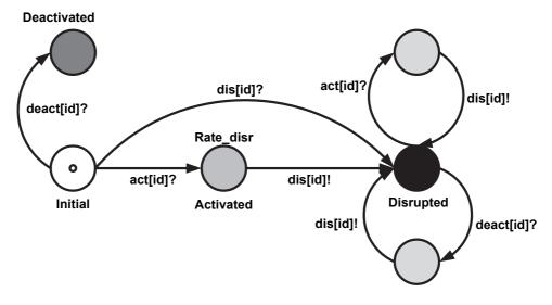
Figure 8. STA template for the DRBD basic block. Here id stands for DRBD block identifier. Here, we consider the disruption of the block is governed by exponential distribution with rate Rate\_disr: $\lambda \in \mathbb{R}_+$ .
