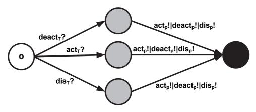
Figure 13. STA template for DRBD SDEP block.
