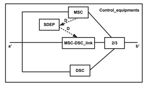
*Figure 6.* DRBD nested in the block of Control\_equipments. The DRBD of the complete system is shown in Figure 5.
