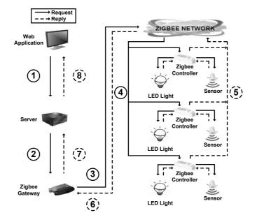
Figure 5. Architecture of Smart Lighting System
