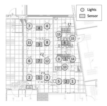
Figure 4. Placement of sensors and lights
