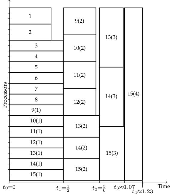
Fig. 3. The schedule of an online algorithm for the lower bound instance with  $\ell = 2$ ,  $K = 4$ , and  $n = 15$  linear chains. The algorithm allocates (approximately) the same number of processors to all linear chains, producing a makespan  $t_4 \approx 1.23$ .
