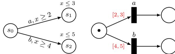
**Fig. 3.** a) A timed automaton  $\mathcal{A}_1$  b) an equivalent timed Petri net
