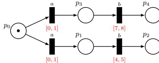
**Fig. 5.** A TPN  $\mathcal{N}_2$  with non-injective labeling.
