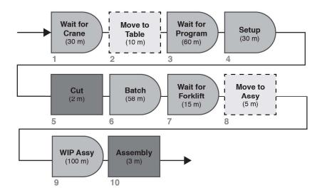
Fig. 4. – Product Path Diagram (Fabrication)
