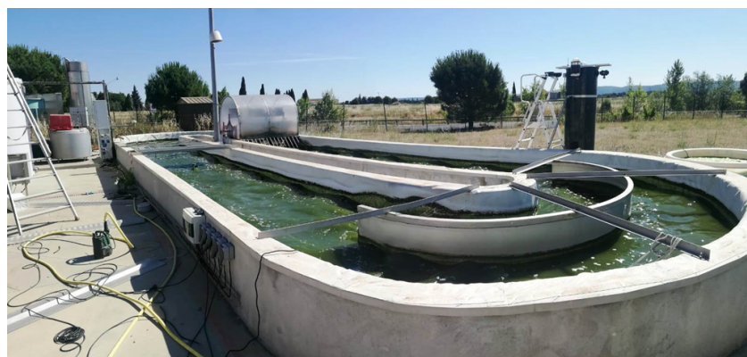
Figure A1. Demonstrative scale raceway with a surface of 56 m 2 , located in the south of France.
