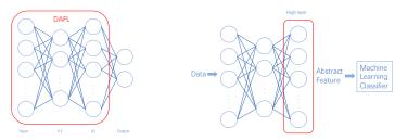
(a) Pre-train DBN model by using (b) Use the remain structure to gen-DAFL erate new feature
