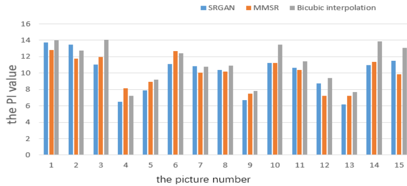
Fig. 10. The reconstruction effect of MMSR compared with SRGAN and Bicubic interpolation. The smaller the value of PI is, the better the visual perception of the result image is.
