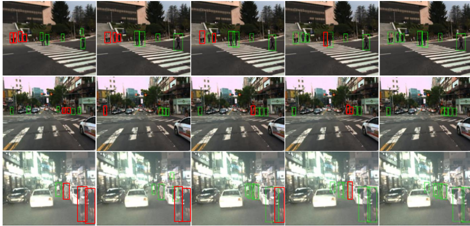
Fig. 4: Comparison of the detection results of existing methods and our method. From left to right are the detection results of ACF-RGB, ACF-RGBT-HOG, CMT-CNN, SDS-RCNN and our method.
