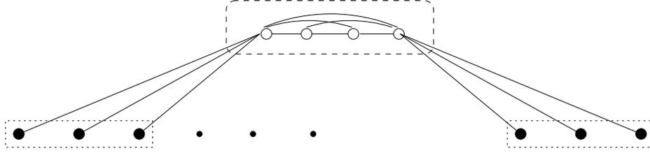
Figure 1: A graph  $G^A$  with a monopoly  $M$  of size  $O(\sqrt{n})$ . (In all our figures, white circles represent vertices of the coalition, and black circles represent vertices controlled by the coalition.)
