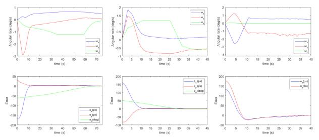
Figure 11: Measured angular rate  $\omega_{\tau}$  and visual feature error for the visual control law in plane (on the left), relief (on the middle) and moving target (on the right) configurations.
