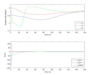
Figure 5: Measured angular rate  $\omega_r$  and visual feature error for the visual control law applied for satellite simulation flying over the port of Brest.
