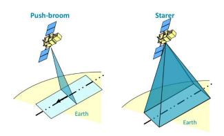
Figure 1:Push-broom and starer technologies
