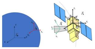
Figure 2: LION mission: a satellite (Fs) directed by its orbital translation and controlled in rotation to track a terrestrial object of interest (Fo) thanks to its camera (Fc). World frame (Fw) is here the equatorial geocentric frame of reference.
