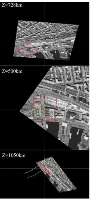
Figure 6: Image trajectory of point **P** and **P**' induced by visual control law in satellite simulation targeting an object of interest in the port of Brest. Satellite motion can be observed as it gets closer to the target, distance to target is reduced from 730km to 500km and both the image and the template are enlarged. After reaching zenith, the satellite moves away. The distance to target increases and the image and the template shrink.
