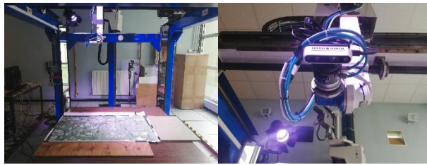
Figure 9: Experimental setup: a satellite image positioned below a Cartesian robot and the Intel D435 camera with a pan-tilt configuration.
