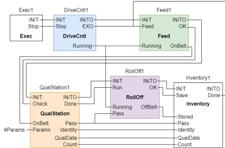
Fig. 4: IEC 61499 application of the conveyor test station
