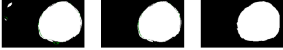
Fig. 4: Example of post-treatment using the rectangular closure. Left: \mathbf{y}^{\text{tgt}} provided by the approach of §3. Center: correction of \mathbf{y}^{\text{tgt}} using rectangular closure. Right: expert segmentation.
