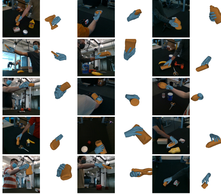
Fig. 7: Qualitative results of our model on the DexYCB benchmark. Our model produces convincing 3D hand-and-object reconstruction results in the real-world setting.
