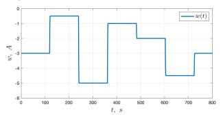
Fig. 4. Loading current w(t) during discharging
