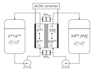
Fig. 1. The configuration of a VRFB system equipped with inlet/outlet open circuit cells
