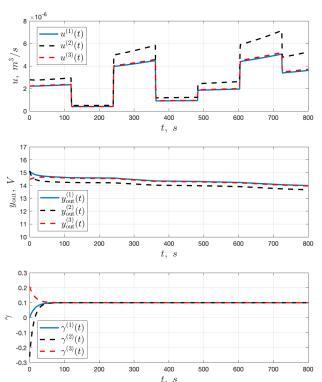
Fig. 5. Evolution of main parameters of the system: flow rate u, outlet OCV  $y_{\text{out}}$ , and the conversion rate  $\gamma$  for three different initial conditions of  $x_1$  and  $x_2$
