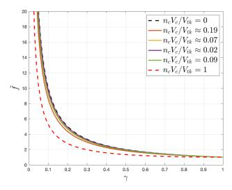
Fig. 3. The plot of  $\tilde{f}$  as a function of the conversion rate  $\gamma \in [0.05, 1]$  for six values of  $n_c V_c / V_{tk}$
