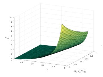
Fig. 2. The behavior of  $\tilde{f}$  depending on the volume ratio and conversion rate,  $n_c V_c / V_{tk} \in [0, 1], \gamma \in [0.1, 1]$
