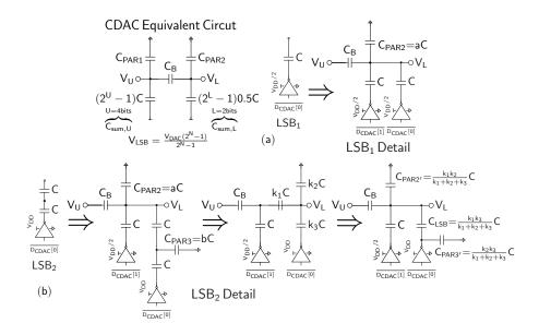
Fig. 5. LSB Capacitor Variation with parasitics: (a) LSB<sub>1</sub>; (b) LSB<sub>2</sub>
