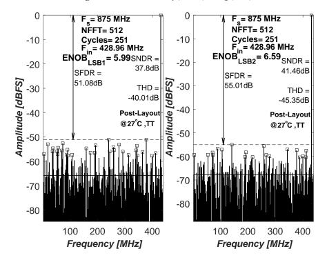
**Fig. 15.** Output Spectrum with 0 dBFS signal applied at 428.96 MHz, sampling frequency is 875 MHz. LSB<sub>1</sub> (left); LSB<sub>2</sub> (right)
