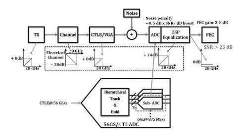
Fig. 1. sub-ADC in a Time Interleaved System
