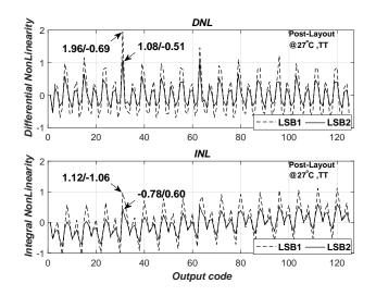
Fig. 14. DNL and INL. LSB<sub>1</sub> (dashed); LSB<sub>2</sub> (solid)
