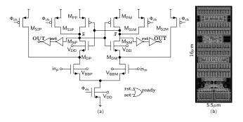
Fig. 7. Strong ARM Comparator: (a) Schematic; (b) Layout
