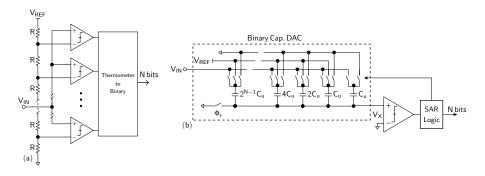
Fig. 2. (a) Flash ADC; (b) SAR ADC with binary-weighted capacitive DAC.
