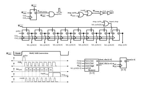
Fig. 11. SAR Logic and timing
