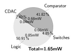
Fig. 12. sub-ADC power consumption breakdown
