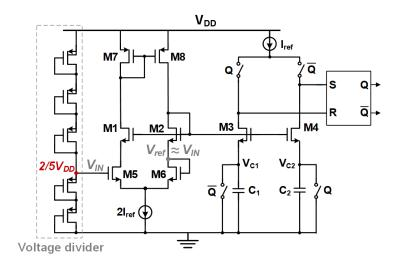
Fig. 3: Proposed voltage sensor.
