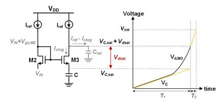
Fig. 10: The delay model and illustrated transition of the source-coupled amplifier transistors (M3 and M4).
