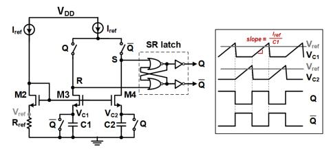
Fig. 1: A dual-phase current-mode relaxation oscillator [6].
