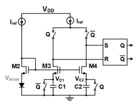
Fig. 4: Proposed temperature sensor. By replacing  $V_{ref}$  with  $V_{diode}$ , a temperature-dependent oscillation is obtained.
