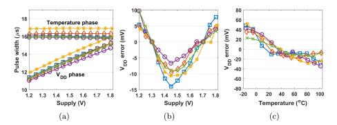
Fig. 15: Measurements of the  $V_{DD}$ -sensitive phase of five hybrid sensor samples, showing (a) pulse width versus  $V_{DD}$ , (b) nonlinearity error after 2-point trimming, and (c) temperature sensitivity.
