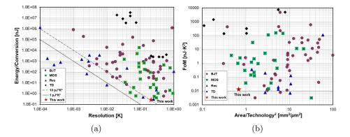
Fig. 13: CMOS smart temperature sensors [14] are compared by plotting (a) energy per conversion versus temperature resolution, and (b) an energy-resolution figure-of-merit (FoM, with unit of  $nJ \cdot K^2$ ) versus normalized circuit area.
