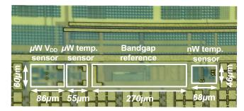
Fig. 12: Die photo of the proposed temperature and voltage sensors, fabricated in 0.18µm CMOS.
