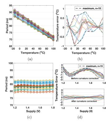
Fig. 16: Measurements of the  $\mu$ W temperature sensor, illustrating (a) oscillation period versus temperature, (b) temperature nonlinearity error after two-point calibration with 15 samples, (c) oscillation period versus  $V_{DD}$ , and (d) supply sensitivity without calibration (upper) and supply sensitivity after curvature correction (lower).
