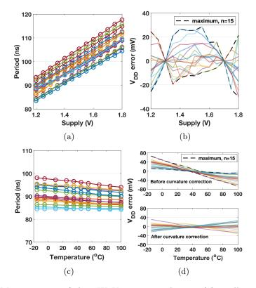
Fig. 17: Measurements of the  $\mu W V_{DD}$  sensor, showing (a) oscillation period versus  $V_{DD}$ , (b)  $V_{DD}$  nonlinearity error, (c) oscillation period versus temperature, (d) temperature sensitivity before (upper) and after curvature correction (lower).
