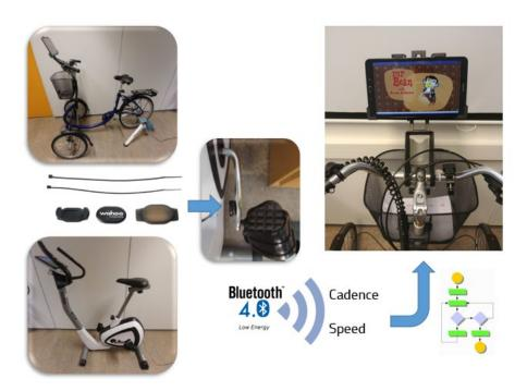
Fig. 1. Set up of the in-door bycycle based activity monitor.
