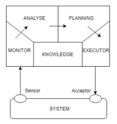
Figure 6: MAPE-K loop for control[10].
