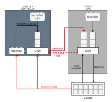
Figure 10: CiGri as an unique controller. Red plain arrows represent the CiGri control loop (even without the added intern controller). The red dotted arrow is additional information. Nothing excludes the possibility of monitoring more information.
