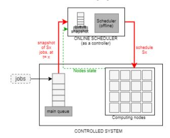
Figure 7: Online scheduler as a controller. Dotted arrows corresponds to possible additional monitoring. Plain arrows constitute the main control loop.
