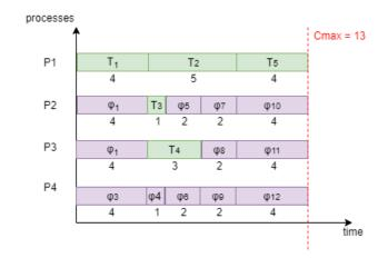
Figure 3: Gantt diagram[1] of the dependency graph in the Figure 1, for n = 4 and  $L = [T_1, T_2, T_3, T_4, T_5]$
