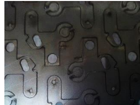
Fig. 2. Detachable metal components in the metal sheet with micro joints
