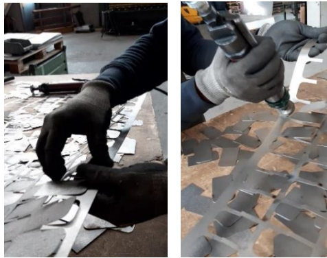
Fig. 4. On the left: manual detaching; on the right: detaching with instrument
