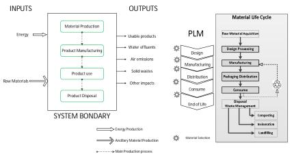
Fig. 2: Using LCA approach for Material life cycle
